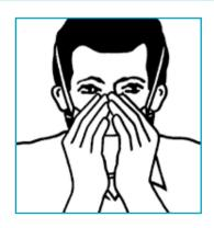
Cover the front of the respirator with both hands, being careful not to disturb the position of the respirator on the face.
